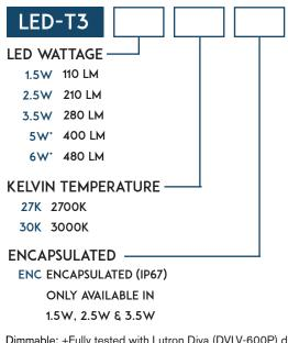
See Encapsulated T3 LED Lamps Spec Sheet for additional details (1.5w, 2.5w, 3.5w only)
