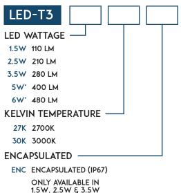
\* <u>Dimmable</u>: +Fully tested with Lutron Diva (DVLV-600P) dimmer and Lightcraft dimmable transformers and LED lamps.
